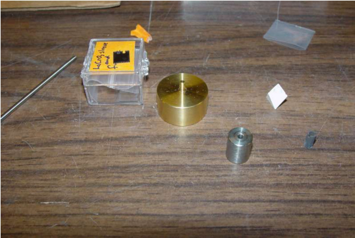
Figure 1: some items of the kit for making the furnace. From left: pin, rhenium foil furnace (on top of plastic box), brass dummy, stainless steel bushing, octahedron, LaCrO 3 sleeve.
