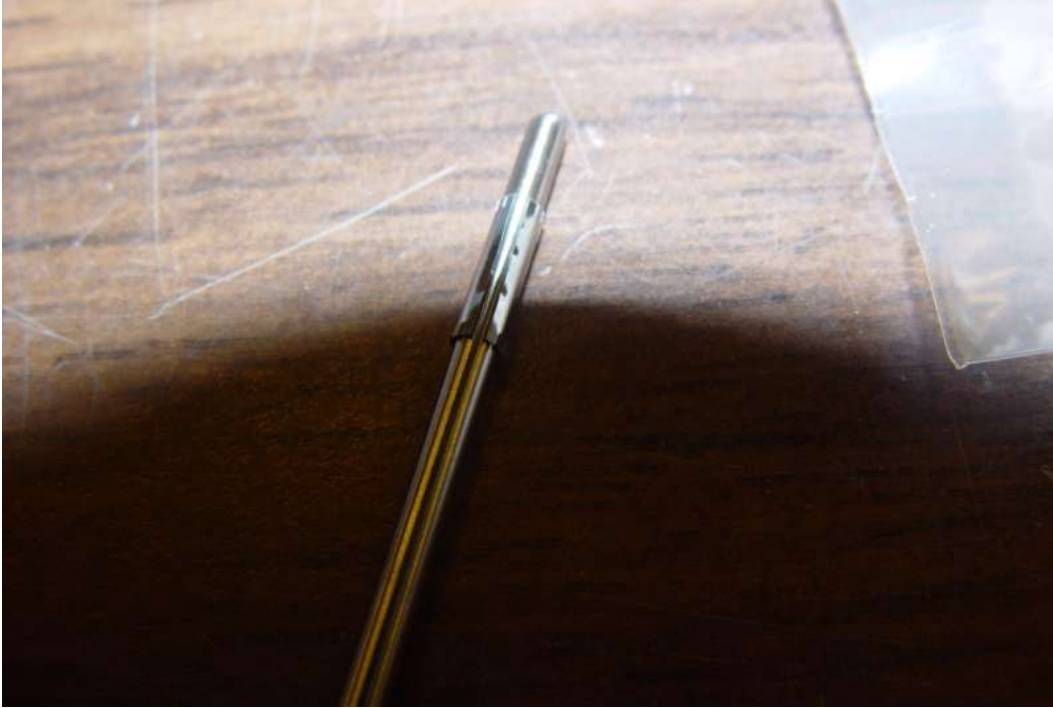
Figure 3. Re furnace wrapped around a drill blank.
