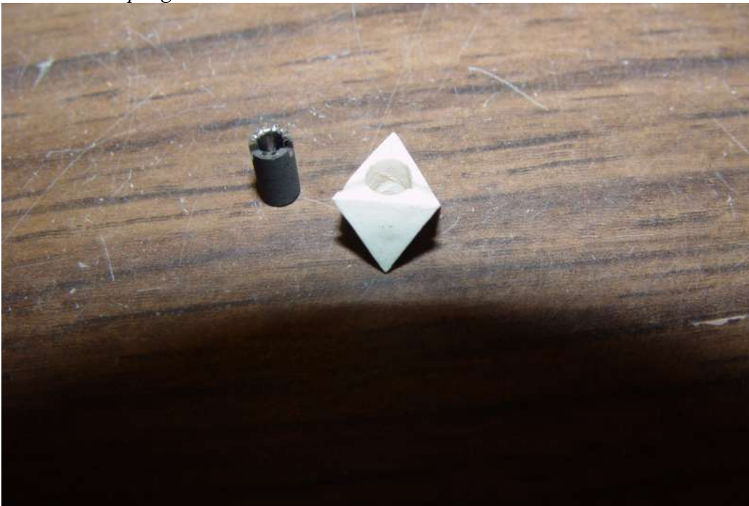
Figure 8: Rhenium furnace in LaCrO 3 sleeve, after all the tabs have been folded outward, also showing the octahedron with thermocouple grooves in it.
