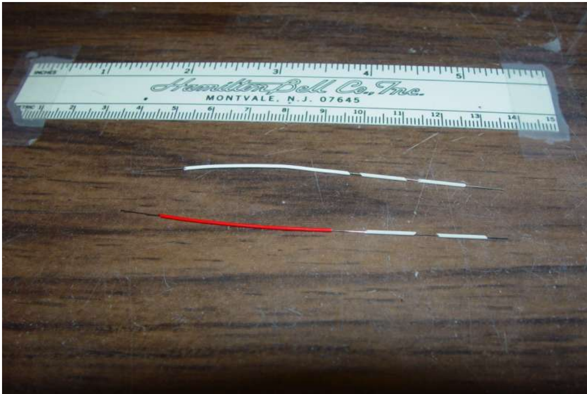
Figure 1. Two legs of a thermocouple with teflon tubing (white and red) and two pieces of mullite tubing on each wire.
